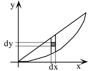
$$x_{CM} = \frac{\int_0^a x dx dy}{\int_0^a dx dy} = \frac{\int_0^a x dx \int_{kx^2}^{cx} dy}{\int_0^a dx \int_{kx^2}^{cx} dy} = \frac{\int_0^a x dx [y]_{kx^2}^{cx}}{\int_0^a dx (cx - kx^2)} =$$
