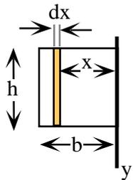
$$I_y = \int_0^b dm x^2 = \int_0^b \sigma ds x^2 = \int_0^b \sigma h dx x^2 = \sigma h \int_0^b x^3 = \sigma h \frac{b^3}{3} = \sigma h b \frac{b^2}{3} = \frac{1}{3} \sigma h b b^2 = \frac{1}{3} m b^2$$
