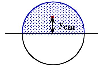
$$A = 1/2 (\pi R^2) \quad y \quad V = 4/3 \pi R^3 \Rightarrow y_G = \frac{V}{2\pi A} = \frac{4/3 \pi R^3}{2\pi \cdot 1/2 \pi R^2} = \frac{4R}{3\pi}$$
