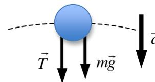
$$\vec{T} + m_1\vec{g} = m_1\vec{a}_1 \Rightarrow T + m_1g = m_1a_1 = m_1\frac{v_{1arriba}^2}{R} \Rightarrow T = m_1\left(\frac{v_{1arriba}^2}{R} - g\right)$$
