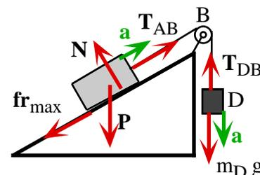
$$T_{AB} - m_A g \text{ sen}30 - fr_{max} = m_A a \Rightarrow (a = \alpha R) \Rightarrow T_{AB} = m_A g \text{ sen}30 + fr_{max} + m_A \alpha R \quad (1)$$
