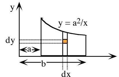
$$\boxed{\int x dA} = \iint x dx dy = \int_a^b x dx \int_0^{a^2/x} dy = \int_a^b x dx \left[ y \right]_0^{a^2/x} = \int_a^b x dx \frac{a^2}{x} = \int_a^b a^2 dx = a^2 \left[ x \right]_a^b = \boxed{a^2(b-a)}$$
