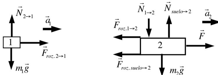
$$\left. \begin{aligned} F_{roz.2 \rightarrow 1} &= m_1 a_1 \\ F - F_{roz.2 \rightarrow 1} - F_{roz.suelo \rightarrow 2} &= m_2 a_2 \\ F_{roz.2 \rightarrow 1} &= \mu N_{2 \rightarrow 1} = \mu m_1 g \\ F_{roz.suelo \rightarrow 2} &= \mu N_{suelo \rightarrow 2} = \mu(m_1 + m_2)g \end{aligned} \right\} \Rightarrow \left\{ \begin{aligned} a_1 &= \mu g \\ a_2 &= \frac{F}{m_2} - \mu \left( \frac{2m_1 + m_2}{m_2} \right) g \end{aligned} \right.$$
