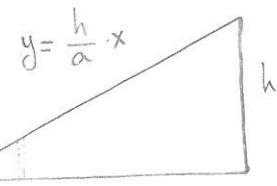
$$x_{CM} = \frac{\int x dA}{\int dA} = \frac{\int_0^a dx \int_0^{(h/a)x} dy \cdot x}{\frac{1}{2}ah} = \frac{\int_0^a dx x \cdot \frac{h}{a} x}{\frac{1}{2}ah}$$
