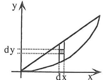
$$\boxed{x_{CM}} = \frac{\iint x \, dx \, dy}{\iint dx \, dy} = \frac{\int_0^a x \, dx \int_{kx^2}^{cx} dy}{\int_0^a dx \int_{kx^2}^{cx} dy} = \frac{\int_0^a x \, dx [y]_{kx^2}^{cx}}{\int_0^a dx [y]_{kx^2}^{cx}} = \frac{\int_0^a x \, dx (cx - kx^2)}{\int_0^a dx(cx - kx^2)} =$$
