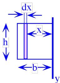
$$I_y = \int_0^b dm x^2 = \int_0^b \sigma ds x^2 = \int_0^b \sigma h dx x^2 = \sigma h \left[ \frac{x^3}{3} \right]_0^b = \sigma h \frac{b^3}{3} = \frac{1}{3} \sigma h b^2 = \frac{1}{3} m b^2$$
