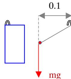
$$0.1mg = 0.4167\alpha \Rightarrow \alpha = \frac{20 \times 9.81 \times 0.1}{0.4167} \frac{\text{rad}}{\text{s}^2} = 47.09 \frac{\text{rad}}{\text{s}^2}$$
