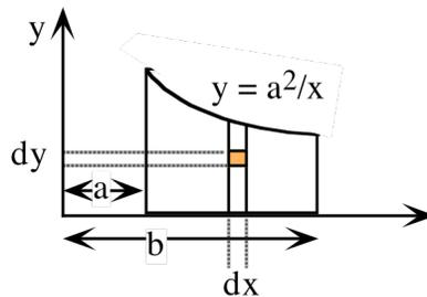
$$\int x \, dA = \iint x \, dx \, dy = \int_a^b x \, dx \int_0^{a^2/x} dy = \int_a^b x \, dx [y]_0^{a^2/x} = \int_a^b x \, dx \frac{a^2}{x} = \int_a^b a^2 \, dx = a^2 [x]_a^b = a^2(b-a),$$
