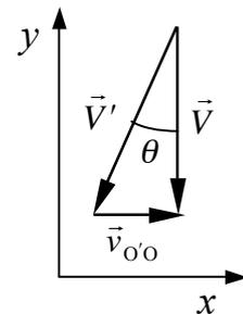
$$\vec{V} = \vec{V}' + \vec{v}_{O'O} \Rightarrow \begin{cases} 0 = -V' \sin \theta + v_{O'O} \\ -V' \cos \theta = -V \end{cases} \Rightarrow \begin{cases} V' = \boxed{57.74 \text{ km/h}} \\ V = \boxed{28.87 \text{ km/h}} \end{cases}$$
