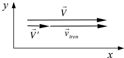
$$V = V' + v_{tren} = \boxed{45 \text{ m/s}}$$
