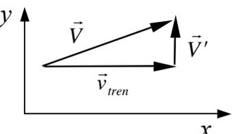
$$V = \sqrt{V'^2 + v_{tren}^2} = \boxed{33.5 \text{ m/s}}$$
