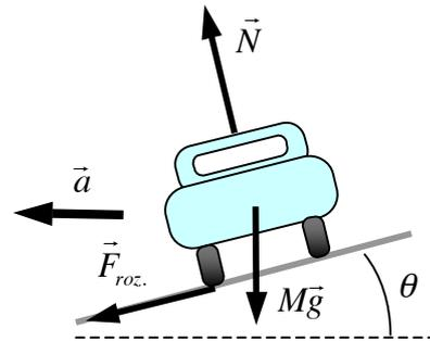
$$\vec{N} + \vec{F}_{\text{roz.}} + M\vec{g} = M\vec{a} \Rightarrow \begin{cases} N \cos\theta - F_{\text{roz.}} \text{sen}\theta - Mg = 0 \\ N \text{sen}\theta + F_{\text{roz.}} \cos\theta = Ma = M \frac{v^2}{R} \end{cases}$$
