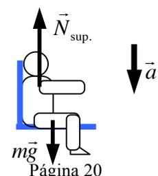
$$\vec{N}_{\text{sup.}} + m\vec{g} = m\vec{a} \Rightarrow mg - N_{\text{sup.}} = ma = m\left(\frac{2\pi}{T}\right)^2 R$$
