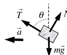
$$\vec{T} + m\vec{g} + \vec{N} = m\vec{a} \Rightarrow \begin{cases} T \text{sen}\theta - N \text{cos}\theta = ma = m\omega^2 R \\ T \text{cos}\theta + N \text{sen}\theta - mg = 0 \end{cases}$$
