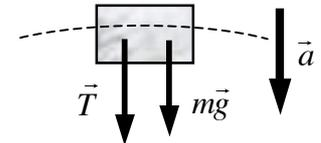
$$\vec{T} + m\vec{g} = m\vec{a} \Rightarrow T + mg = ma = m\frac{v^2}{R} \Rightarrow T = m\left(\frac{v^2}{R} - g\right)$$
