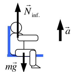
$$\vec{N}_{\text{inf.}} + m\vec{g} = m\vec{a} \Rightarrow N_{\text{inf.}} - mg = ma = m \left( \frac{2\pi}{T} \right)^2 R$$
