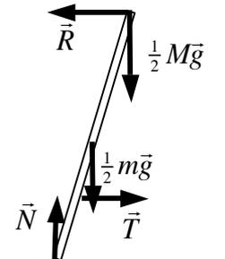
$$\Rightarrow \left(\frac{1}{2}mg\right)\left(\frac{L}{2}\right)\sin\left(\frac{\varphi}{2}\right) + T\left[L\cos\left(\frac{\varphi}{2}\right) - h\right] - NL\sin\left(\frac{\varphi}{2}\right) = 0$$
