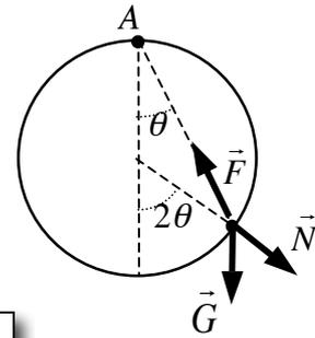
$$\sum_i \vec{F}_i = 0 \Rightarrow \left\{ \begin{array}{l} F \cos \theta - N \cos 2\theta - G = 0 \\ N \sin 2\theta - F \sin \theta = 0 \end{array} \right\} \Rightarrow \left\{ \begin{array}{l} N = G \\ \cos \theta = \frac{F}{2G} \end{array} \right.$$
