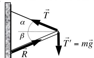
$$\sum_i \vec{F}_i = 0 \Rightarrow \left\{ \begin{array}{l} R \cos\beta - T \cos\alpha = 0 \\ R \text{sen}\beta + T \text{sen}\alpha - mg = 0 \end{array} \right\} \Rightarrow \left\{ \begin{array}{l} T = \frac{mg}{\cos\alpha(\text{tg}\alpha + \text{tg}\beta)} \\ R = \frac{mg}{\cos\beta(\text{tg}\alpha + \text{tg}\beta)} \end{array} \right.$$
