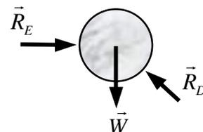
$$\left. \begin{aligned} R_E - R_D \cos \varphi &= 0 \\ R_D \sin \varphi - W &= 0 \end{aligned} \right\} \Rightarrow \left\{ \begin{aligned} R_D &= \frac{W}{\sin \varphi} \\ R_E &= \frac{W}{\operatorname{tg} \varphi} \end{aligned} \right.$$
