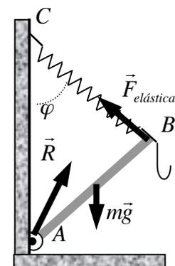
$$F_{elástica}L - mg\left(\frac{L}{2}\right)\sin\varphi = 0 \Rightarrow k\Delta l = \frac{1}{2}mg\sin\varphi$$
