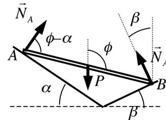
$$\Rightarrow \begin{cases} N_A = \frac{mg}{\text{cos } \alpha + \frac{\text{sen } \alpha}{\text{tg } \beta}} \\ N_B = \frac{mg}{\text{cos } \beta + \frac{\text{sen } \beta}{\text{tg } \alpha}} \end{cases}$$
