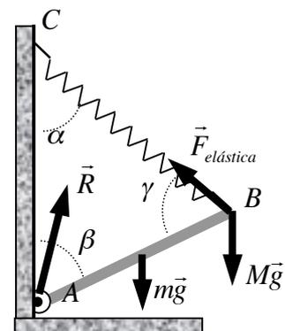
$$\left. \begin{array}{l} l\sin\alpha = L\sin\beta \\ l\cos\alpha = \sqrt{2}L - L\cos\beta \end{array} \right\} \Rightarrow \operatorname{tg}\alpha = \frac{\sin\beta}{\sqrt{2} - \cos\beta} \Rightarrow \alpha = 43.45^\circ$$
