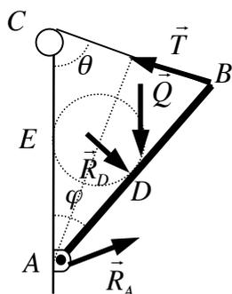
$$\left. \begin{aligned} R_{A,x} + R_D \cos \varphi - T \sin \theta &= 0 \\ R_{A,y} - R_D \sin \varphi + T \cos \theta - Q &= 0 \\ T(2L) \sin \theta - QL \sin \varphi - R_D \overline{AD} &= 0 \end{aligned} \right\}$$
