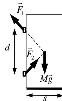
$$F_1 \sin \varphi = F_2 \sin \varphi = \frac{1}{2} Mg \Rightarrow \boxed{F_1 = F_2 = 353.3 \text{ N}}$$
