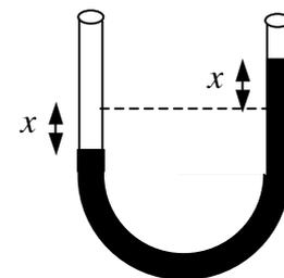
$$E_{pot.grav.} = \Delta m_{líquido} g x = \Delta V_{líquido} \rho g x = (\pi R^2 x) \rho g x = \frac{1}{2} (2\pi R^2 \rho g) x^2$$
