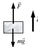
$$M\vec{g} + \vec{F} = M\vec{a} \Rightarrow Mg - F = Ma_x \left. \vphantom{M\vec{g} + \vec{F} = M\vec{a}} \right\} \Rightarrow F = M \left( g + \frac{v}{\Delta t} \right) = \boxed{0.148 \text{ N}}$$
