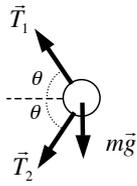
$$\left. \begin{aligned} (T_1 + T_2)\cos\theta &= m\omega^2 L \cos\theta \\ (T_1 - T_2)\sin\theta - mg &= 0 \end{aligned} \right\}$$
