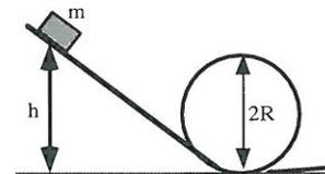
$$mgh = m g 2R + \frac{1}{2}mv_{\text{fin}}^2 \Rightarrow K_{\text{fin}} = \frac{1}{2}mv_{\text{fin}}^2 = mg(h - 2R).$$
