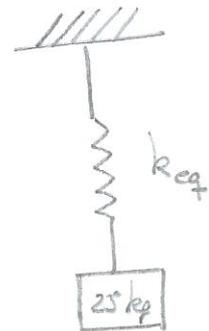
$$(a) \Rightarrow T = 2\pi \sqrt{\frac{m}{k}} = 2\pi \sqrt{\frac{25 \text{ kg}}{3692 \text{ N/m}}} = 0,517 \text{ s}$$
