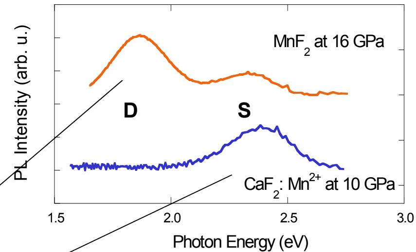
PL lifetime in  $\text{CaF}_2 : \text{Mn}^{2+}$  ( $\tau = 14$  ms) is bigger than in  $\text{MnF}_2$  (4 ms >  $\tau > 2$  ms)
