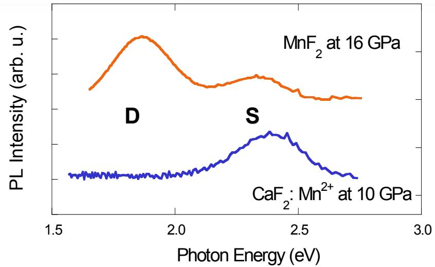
PL lifetime in  $\text{CaF}_2$ :  $\text{Mn}^{2+}$  ( $\tau = 14$  ms) is bigger than in  $\text{MnF}_2$  ( $4 \text{ ms} > \tau > 2 \text{ ms}$ )
