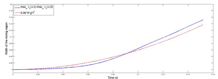
Comparison between the  $z$ -model (blue) and the empirical value (red) for the width of the mixing region [1]
