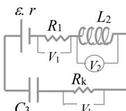
Impedancia:  $Z = \sqrt{\left(\sum_k R_k\right)^2 + \left(\sum_k \left[L_k \omega - \frac{1}{C_k \omega}\right]\right)^2} = \sqrt{R^2 + \left(L\omega - \frac{1}{C\omega}\right)^2}$
