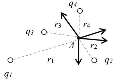
Relación campo-potencial:  $\vec{E} = -\text{grad } V = -\left(\frac{\partial V}{\partial x} \vec{i} + \frac{\partial V}{\partial y} \vec{j} + \frac{\partial V}{\partial z} \vec{k}\right)$
