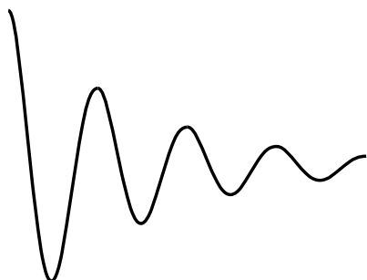
c / The amplitude is halved with each cycle.
