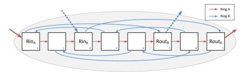
Fig. 4: Paths of two disjoint Hamiltonian rings in a group of a dragonfly network with h = 4. The remaining links have been omitted for simplicity
