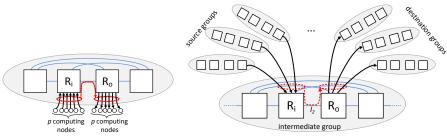
(a) Saturation under traffic local to a (b) Pathological saturation of the single local link,  $l_2$ , connect-group ing  $R_i$  and  $R_o$  in the intermediate group.
