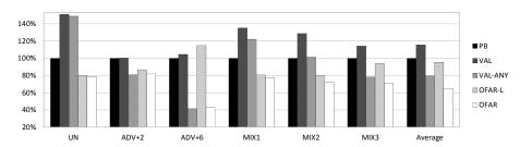
Fig. 8: Burst consumption time, normalized to PB, using 3/2 VCs. Lower is better
