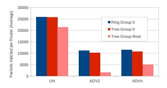
Fig. 12: Average number of packets injected per router in groups 0 and *Root* with an offered load of 1 phit/(node  $\cdot$  cycle), when BCM and only 2/1(+1) VCs are used
