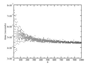
Unitary time spent (time per node and corresponding weight) in seconds as a function of the degree
