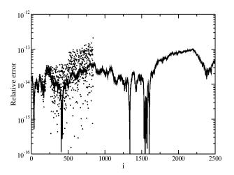
Relative error in the computation of scaled weights (solid line) and unscaled weights (dots) for the 5000-point Gauss Hermite formula as a function of i, with i numbering the positive nodes in increasing order.
