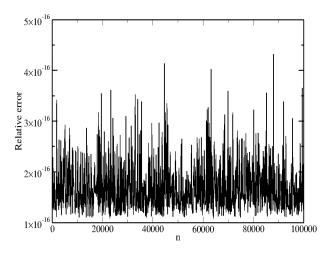
Maximum relative error in the computation of the nodes as a function of the degree n
