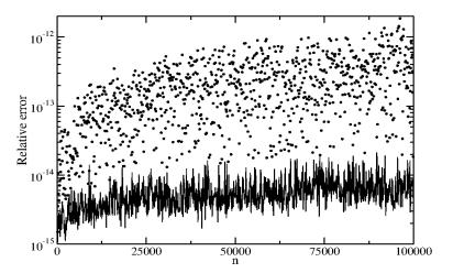
Maximum relative errors in the computation of the nodes for *n*-point Gauss–Laguerre quadrature with  $\alpha = 0$  (dots). We also show the maximum error when it is evaluated only for the nodes for which the weights are larger than  $10^{-30}$  (solid line); the error in this case is smaller.
