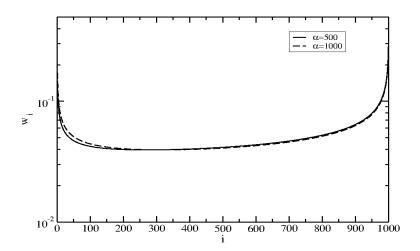
Gauss-Laguerre doubly-scaled weights as a function of the number i of the nodes  $x_i$  ( $x_0 < x_1 < \cdots$ ), where the degree is n = 1000. Two values of  $\alpha$  are considered:  $\alpha = 500$  and  $\alpha = 1000$
