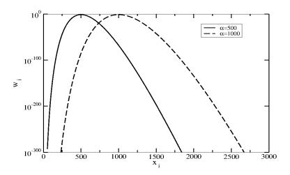
Gauss-Laguerre weights as a function of the nodes  $x_i$ , where the degree is n=1000. Two values of  $\alpha$  are considered:  $\alpha=500$  and  $\alpha=1000$
