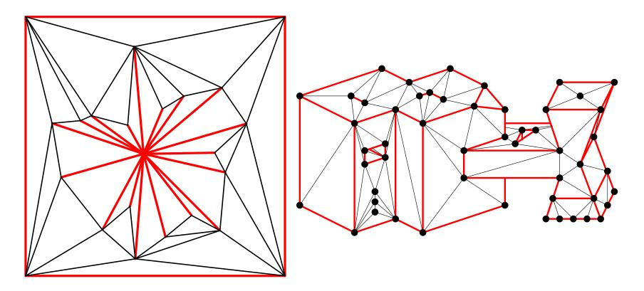
The constrained Delaunay triangulation is the union of all constrained Delaunay simplices, *if* the union is a triangulation. In 3D, a PLC might have no CDT. What is "constrained Delaunay" in 3D?
