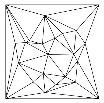
Delaunay triangulation of vertices might not conform to constraining segments.
