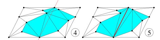
Slowly lift vertices according to distance from new segment. Maintain lower convex hull as we go, using bistellar flips.
