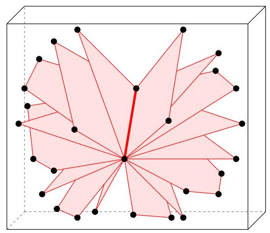
It is difficult to mesh the interior of this box with Delaunay tetrahedra. A new vertex inserted in one facet tends to knock out triangular faces in adjacent facets.
