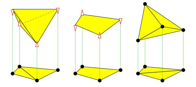
As the lifted vertices move vertically, use flips to maintain the lower convex hull.
