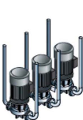
3 in-line pumps in parallel limited maintenance access because of pipework
