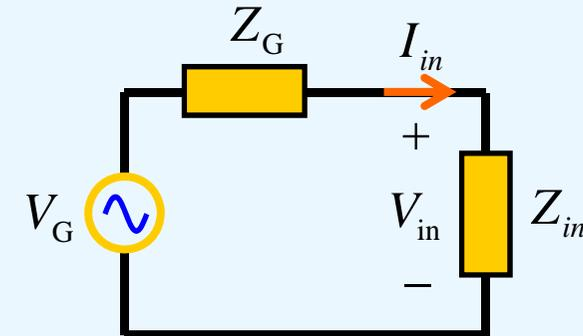
$$V_{in} = V_g \frac{Z_{in}}{Z_g + Z_{in}}$$
