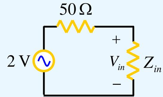
$$V_{in} = 2 \frac{100}{150} = \frac{4}{3} \text{ V}$$
