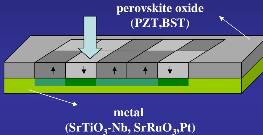
The use as a NV-FRAM depends on the existence of a polar ground state ...
