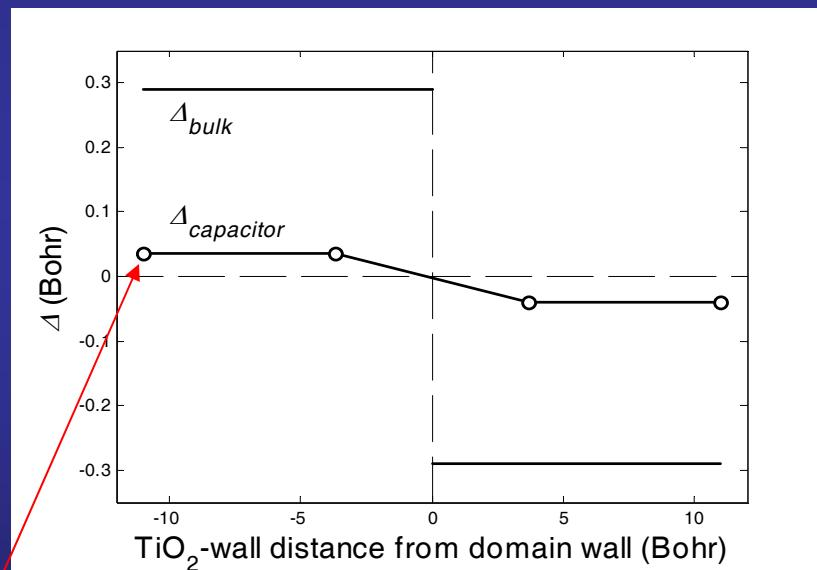
About 1/10 of bulk soft-mode polarization
