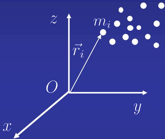
$$\vec{r}_{\text{CM}} = \frac{\sum_{i=1}^n m_i \vec{r}_i}{\sum_{i=1}^n m_i} = \frac{\sum_{i=1}^n m_i \vec{r}_i}{M}$$
