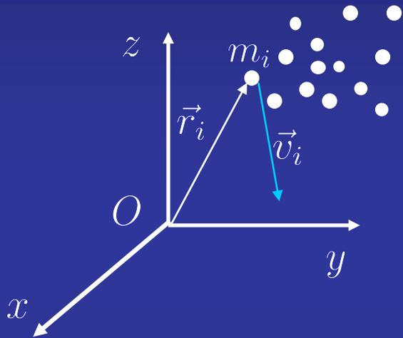
$$\vec{v}_{\text{CM}} = \frac{d\vec{r}_{\text{CM}}}{dt} = \frac{1}{M} \sum_{i=1}^n m_i \frac{d\vec{r}_i}{dt} = \frac{1}{M} \sum_{i=1}^n m_i \vec{v}_i$$
