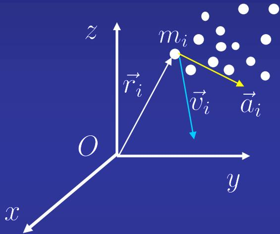
$$\vec{a}_{\text{CM}} = \frac{d\vec{v}_{\text{CM}}}{dt} = \frac{1}{M} \sum_{i=1}^n m_i \frac{d\vec{v}_i}{dt} = \frac{1}{M} \sum_{i=1}^n m_i \vec{a}_i$$
