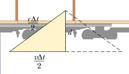
$$\Delta t = \frac{\Delta t_p}{\sqrt{1 - \frac{v^2}{c^2}}} = \gamma \Delta t_p \qquad \qquad \gamma = \frac{1}{\sqrt{1 - \frac{v^2}{c^2}}}$$
