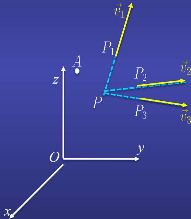
$$\begin{aligned}\vec{M}_A &= \sum_{i=1}^n \vec{AP}_i \times \vec{v}_i = \sum_{i=1}^n (\vec{AP} + \vec{PP}_i) \times \vec{v}_i \\ &= \sum_{i=1}^n \vec{AP} \times \vec{v}_i + \sum_{i=1}^n \vec{PP}_i \times \vec{v}_i \\ &= \vec{AP} \times \sum_{i=1}^n \vec{v}_i + 0 \\ &= \vec{AP} \times \vec{R}\end{aligned}$$
